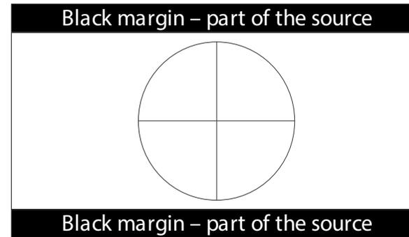
If we change the setting to TheaterScope, the black lines will disappear but the image will stretch vertically to reach the top and bottom of the DMD™:
